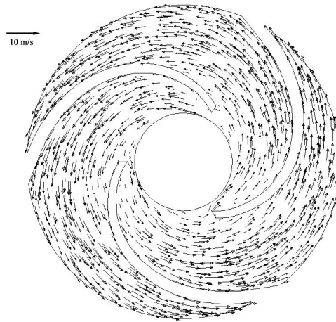
Fig. 2 the relative velocity field in the impeller central-symmetrical faces
